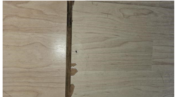
18 Close view of failed joint and panel
