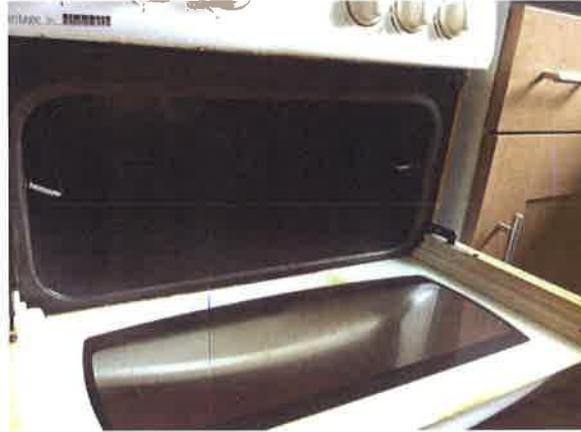
3. Grill with broken runner and missing seal
