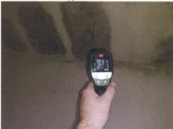
3 Recording of environmental readings – below dewpoint.
