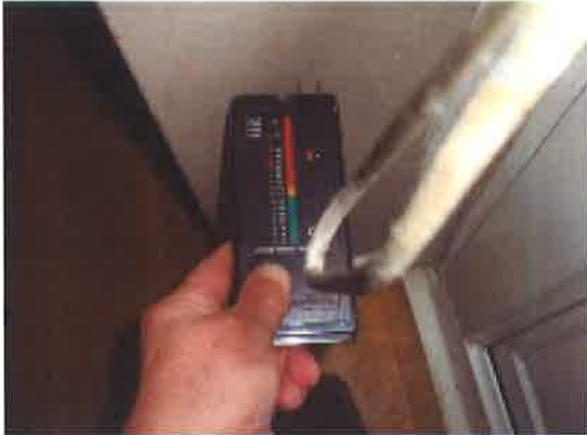
DAMP READINGS AT FRONT ENTRANCE DOOR
