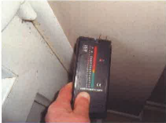
DAMP READINGS AT FRONT ENTRANCE DOOR
